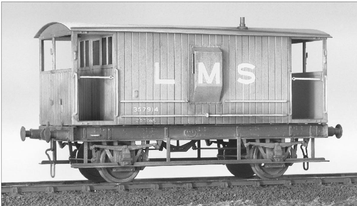
**Prototype.** 950 vehicles were built between 1927 and 1931 .They lasted well into BR days. As they got older and more Dilapidated extra strapping was applied and this is included in the kit .
